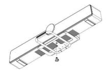
Open the camera clip bracket and place it on top of the display. Make sure that it's firmly attached.
