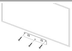
Securely mount the KAC-BAR-81 by hanging the wallmounting bracket onto the hook bracket. Make sure that it's firmly attached.
