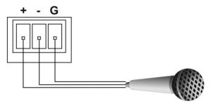
Figure 6: Connecting a microphone
