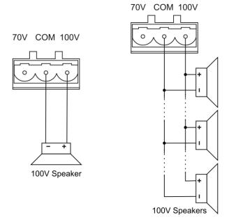
Figure 4: Connecting One or Multiple Speakers to the 920 (100V)
