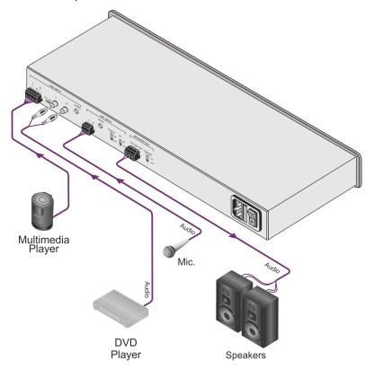
Figure 3: Connecting the 920 Power Amplifier
