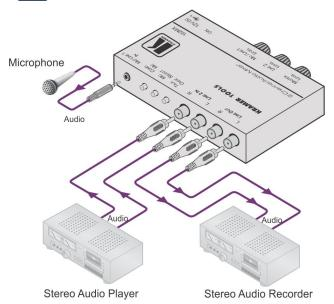
Figure 2: Connecting the 102MX 2 Channel Audio Mixer
